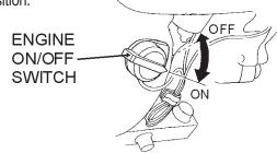
Figure 20. Engine ON/Off Switch
